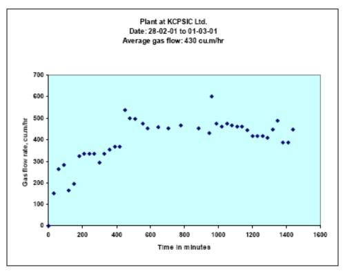
Fig 5. Typical plant loading of Hydrogen sulphide scrubbing system
