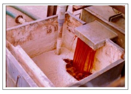
Fig 3. Scrubbing Solution used & Precipitated Sulphur produced by ISET Process
