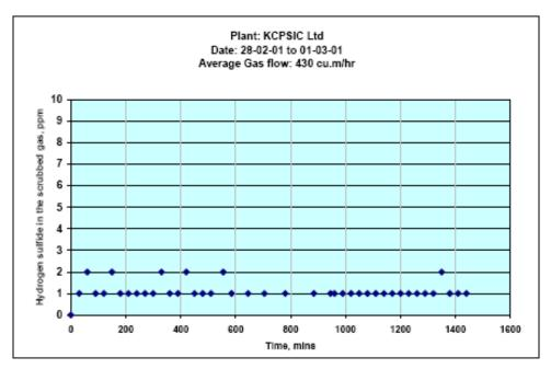
Fig 4. Performance of the hydrogen sulphide scrubbing system at average gas flow rate of 430 m<sup>3</sup>/hr
