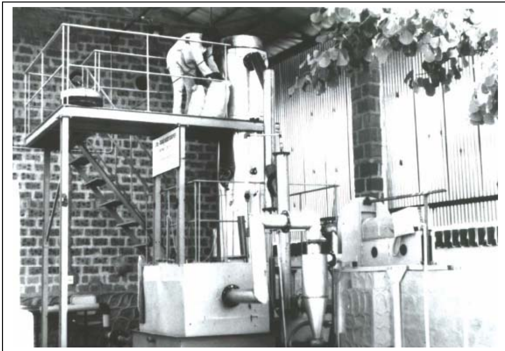
A 100 kWe Gasifier in service of electricity needs of a Paper Industry at JHANSI
