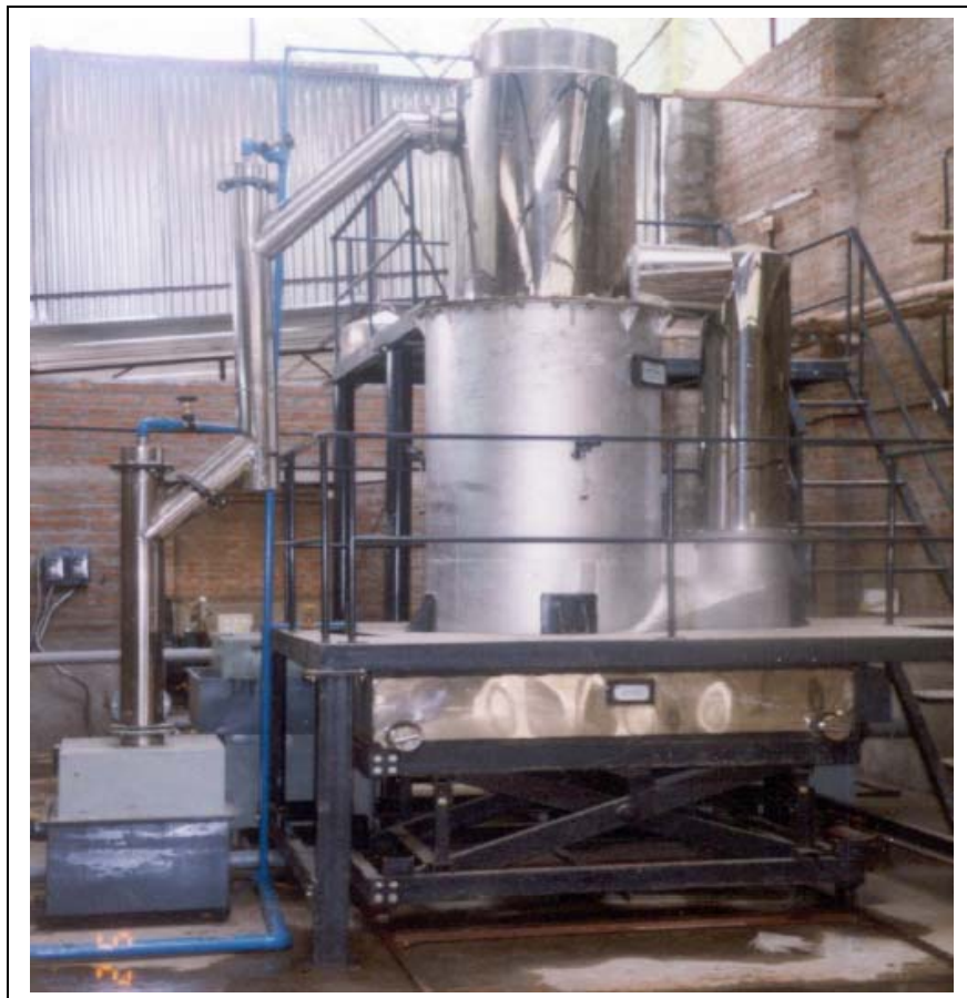
50 kg/hr gasifier at Bethmangala, Kolar
