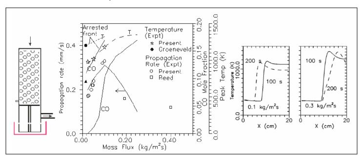
With increase in mass flux the front velocity initially increases and then reduces
