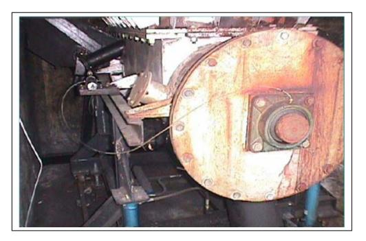
The reactor bottom was modified to accommodate a screw system inplace of the earlier water seal design. This facilitated intermittent char/ash extraction. Since the screw extractor is housed in the pit, the ash/char disposed by the screw in the pit needs to be disposed off at theground level. This is done by using an ash conveyor. The char/ash is finally disposed off at ground level using a combination of char/ash conveyor and manually operated bucket elevator
