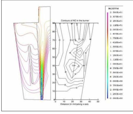
The average NOx emissions at the exhaust are ~12 ppm. EINOx  $\approx$ 21 g/kg of fuel
