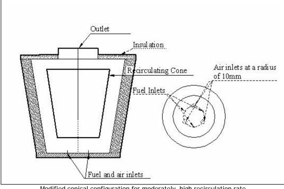
Modified conical configuration for moderately high recirculation rate and larger heat release rates
