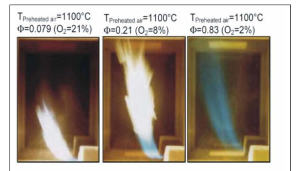
Propane flame photographs with combustion air temperature of 1100°C and O<sub>2</sub> conc. (from left to right) of 21%, 8% and 2% (Nitrogen as the dilution gas).
