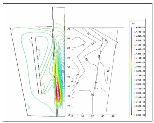
Computed and measured Oxygen contours in the burner
