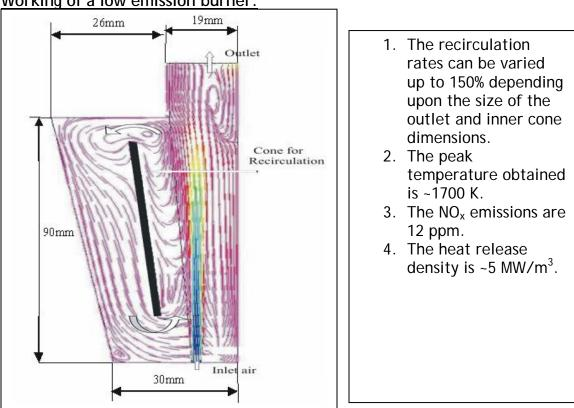
Working of a low emission burner:
