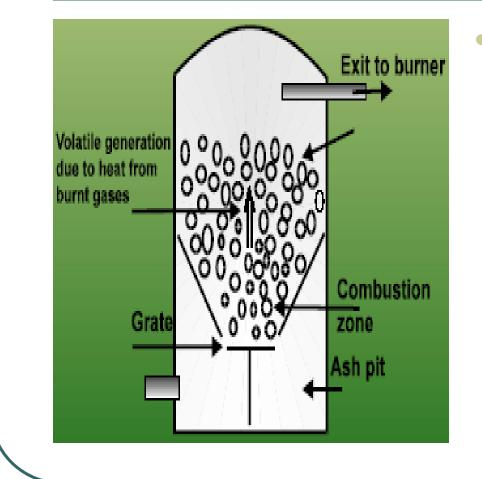
The combustible gases at the exit have a large amount of volatiles. If the combustible gases are cooled to ambient temperature, the tar in the gas condenses and leads to problems of blockage. The gas is fit for direct use in burners. This technique is useful if the downdraft kind cannot be used. It has been used for waste contaminated wood.
