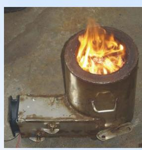
Staged air addition with separate controls for primary and secondary air
