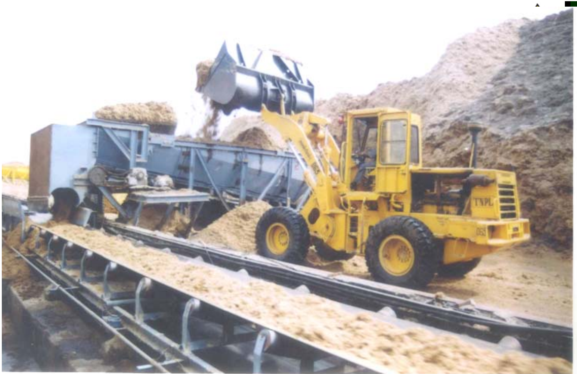
FEEDING OF BAGASSE IN THE CONVEYOR BY FRONT END LOADER
