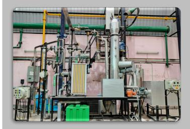
Oxy-steam gasification technology using gasifying oxygen and steam as the media, converts solid biomass to hydrogenrich syngas (a mixture of  $H_2$ , CO,  $CH_4$  and  $CO_2$ gases). With surplus biomass from agro & forest residues (120 - 150 MMT) and municipal solid waste (62 Mt) generated annually. this technology holds great potential in meeting the no/low-carbon hydrogen demands of the future.
