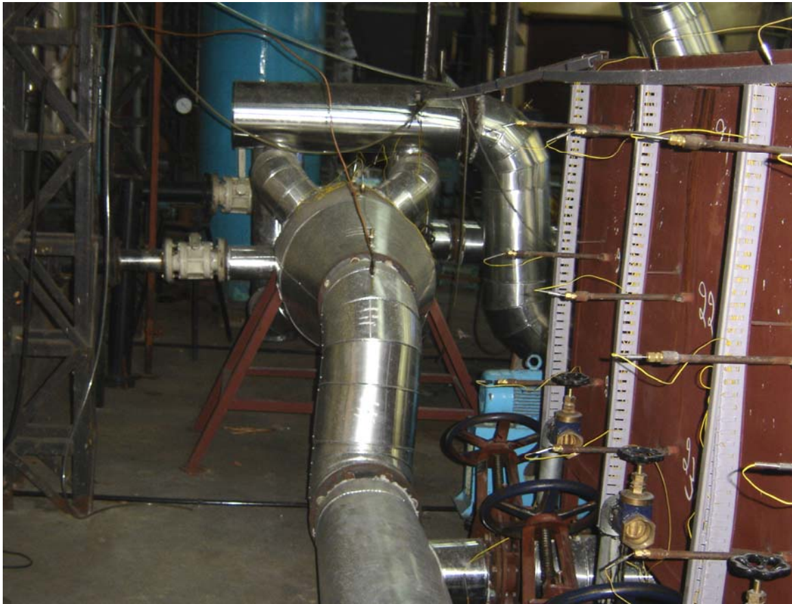
Plate 10: Thermocouple instrumentation on the Torrefaction Chambers
