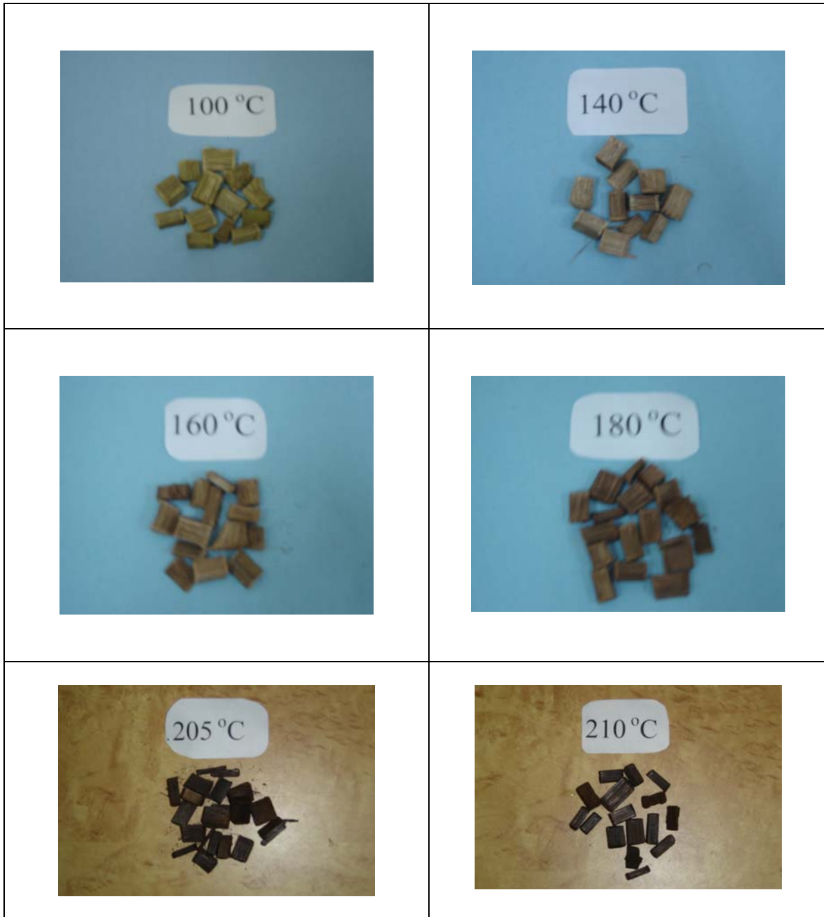
Plate 2: Bamboo samples during various stages of heating. At about 205° C the bamboo loses its tenacity and becomes brittle, indicating bamboo is torrefied
