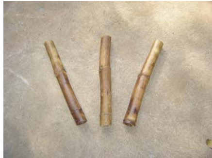
Bamboo Post-drying at 100° C
