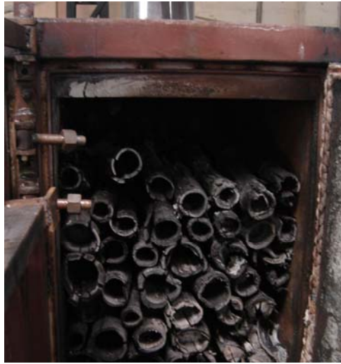
Plate 11: Torrefied Bamboo from the Test Plant
