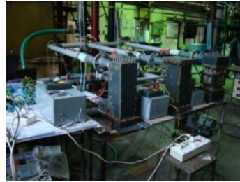
Plate-Wire, Plate-Plate and Cylinder-Wire ESPs, in a Parallel Test
