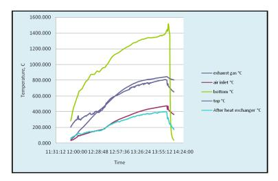
Temperature profile on the insulated burner with recuperator
