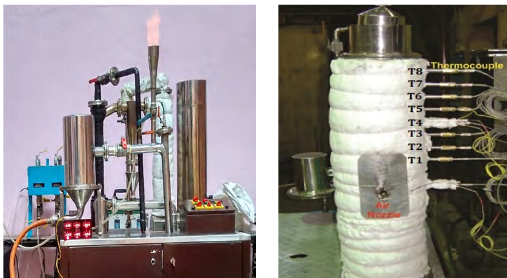
Fig 2.2 Gasifier (3kg/hr) with 103 mm diameter reactor
