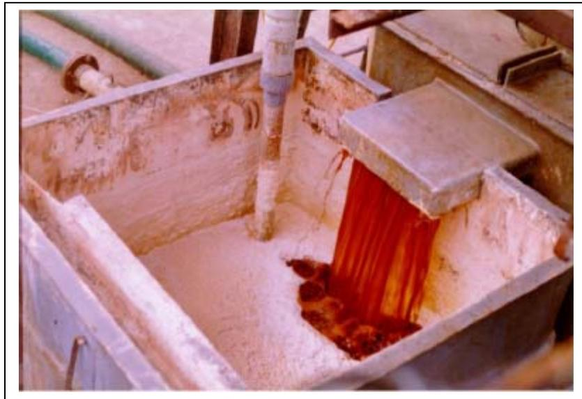
Fig 3. Scrubbing Solution used & Precipitated Sulphur produced by ISET Process
