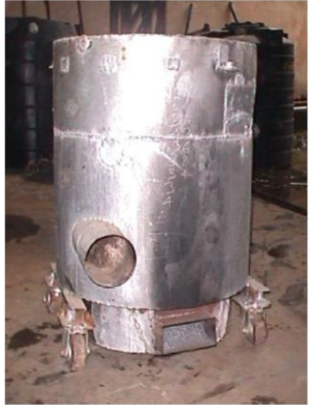
Industrial scale Gasifier stove( ~25kWth )
