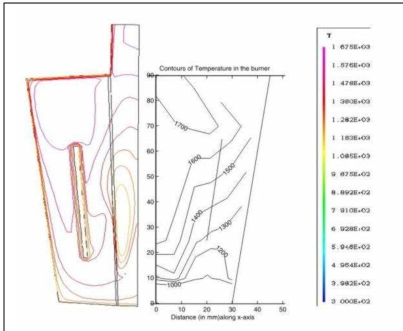
Fig. Measured and predicted temperature profiles
