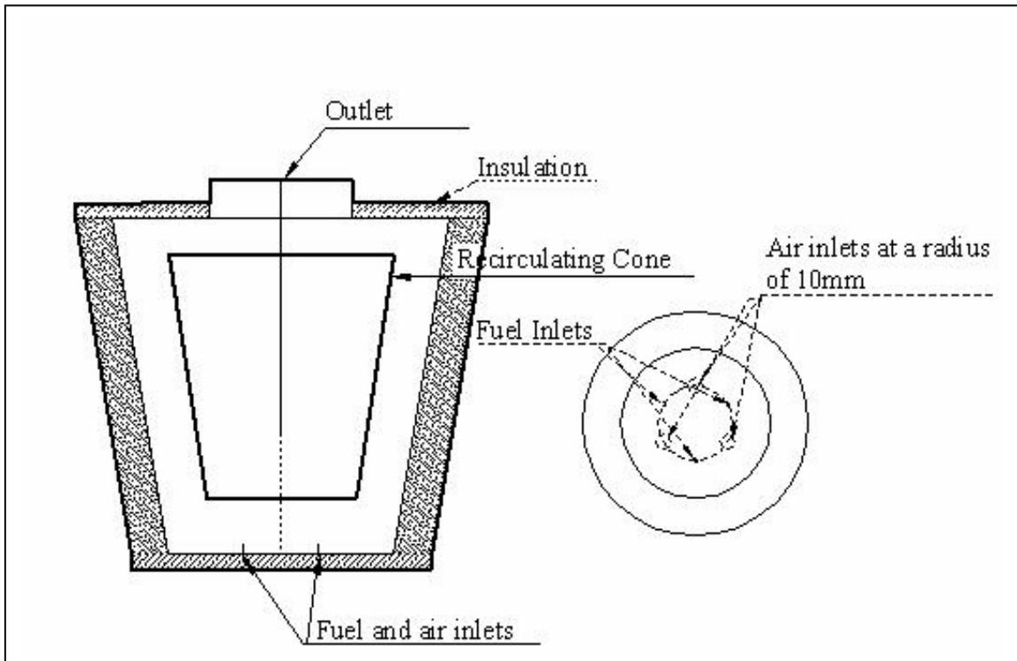
Modified conical configuration for moderately high recirculation rate and larger heat release rates
