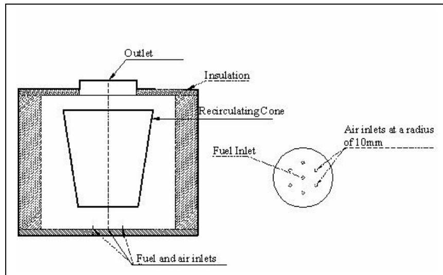
A proposed cylindrical configuration for moderately high recirculation
