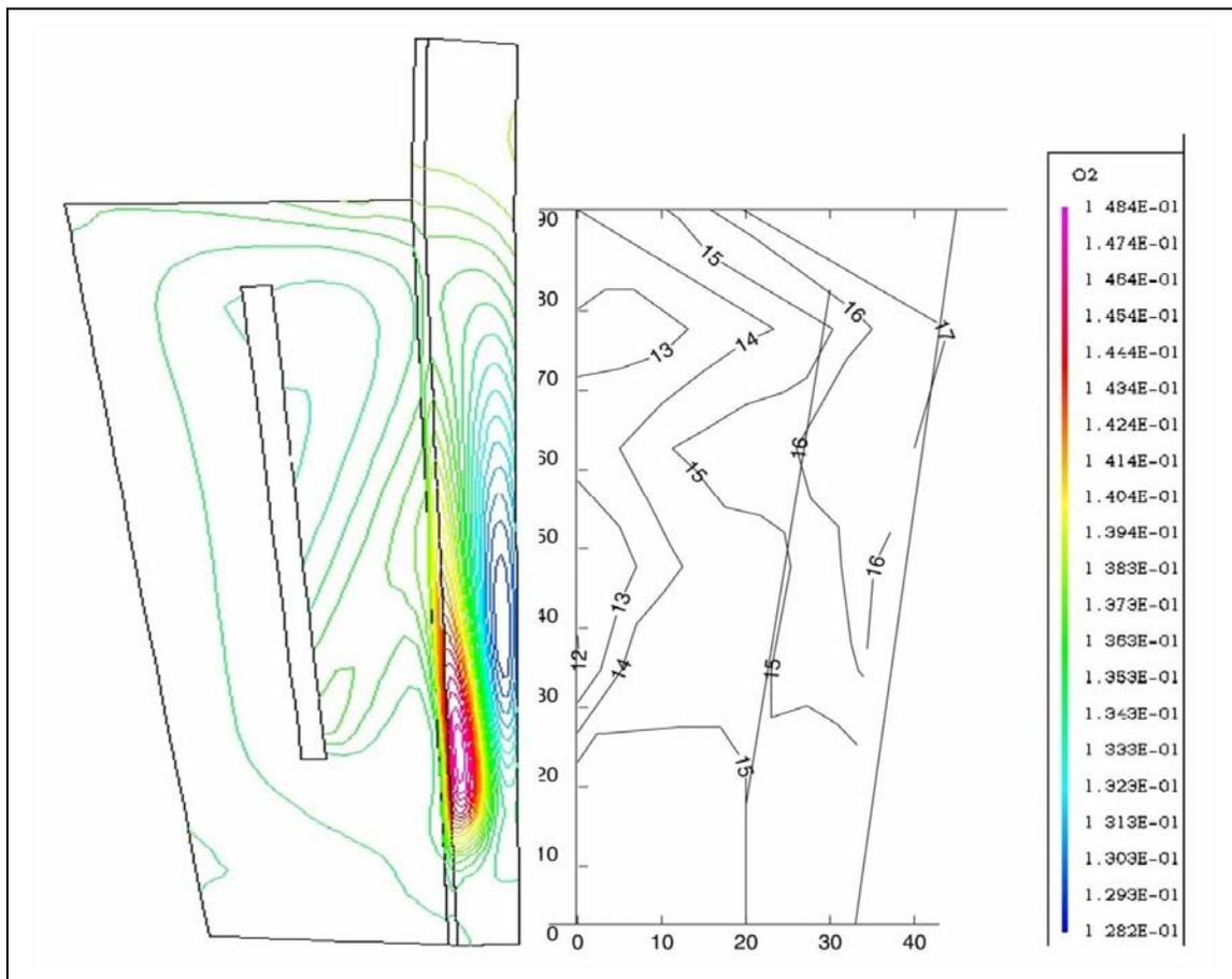
Computed and measured Oxygen contours in the burner
