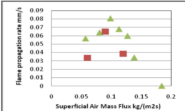
Flame Propagation rate for wood and coconut shells at different flux
