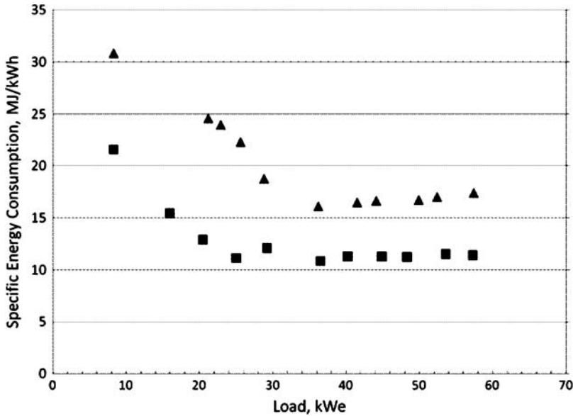
Figure 5. SEC in diesel and dual fuel modes.
