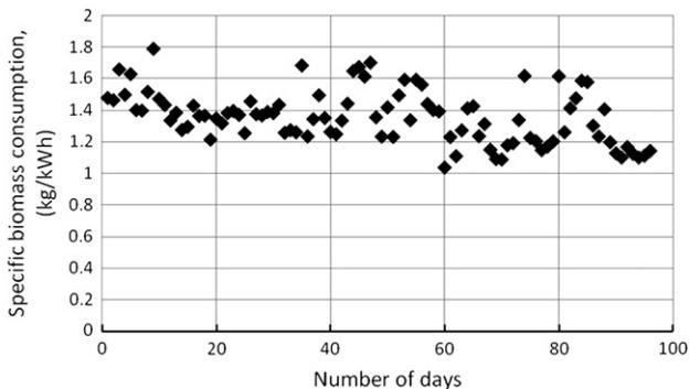
Fig. 9. Specific fuel consumption over 2000 h of operation.
