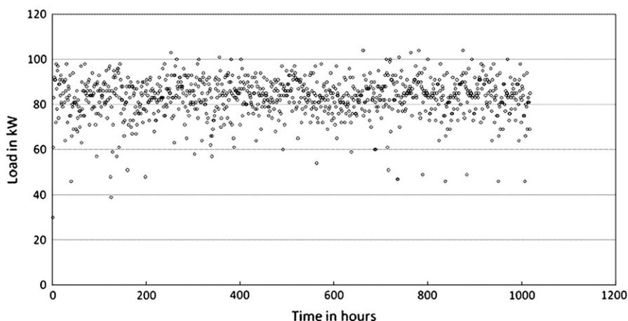
Fig. 7. Electricity generated during the 1000 h of operation.
