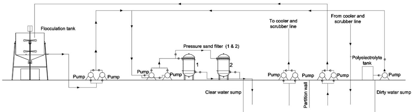
Fig. 6. Block diagram of the water treatment process.
