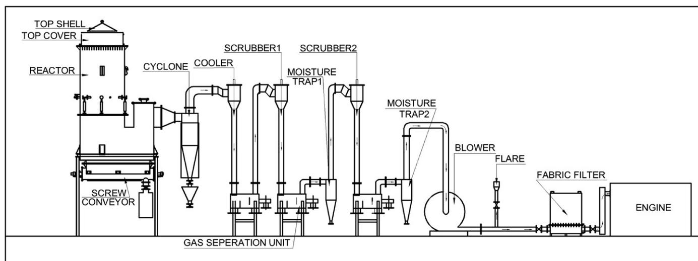
Fig. 1. Schematic of the biomass gasification plant.
