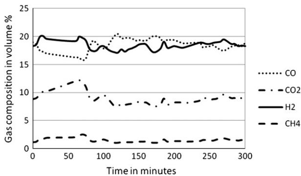
Fig. 5. Producer gas composition at a load of 90 kW.
