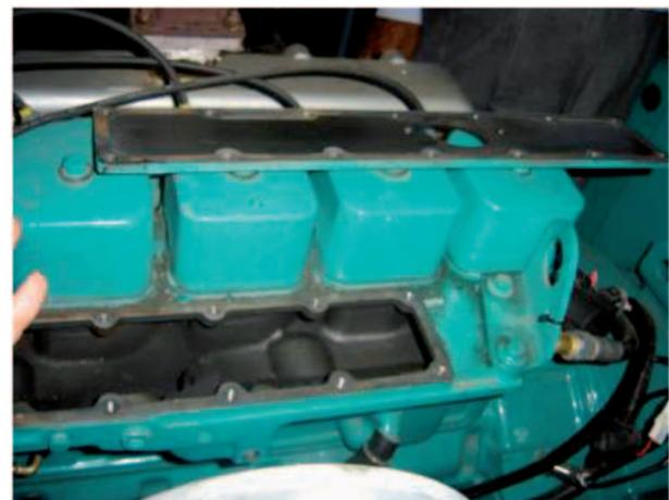
Fig. 6 Intake manifold at the completion of 100 hours
