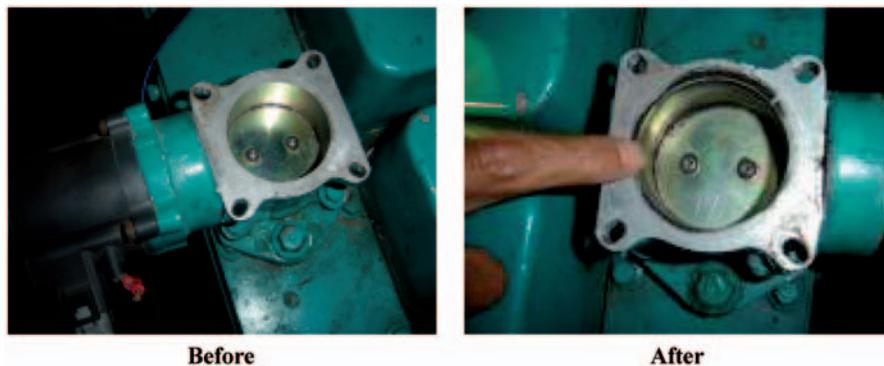
Fig. 5 Throttle valve before and after 100 hours
