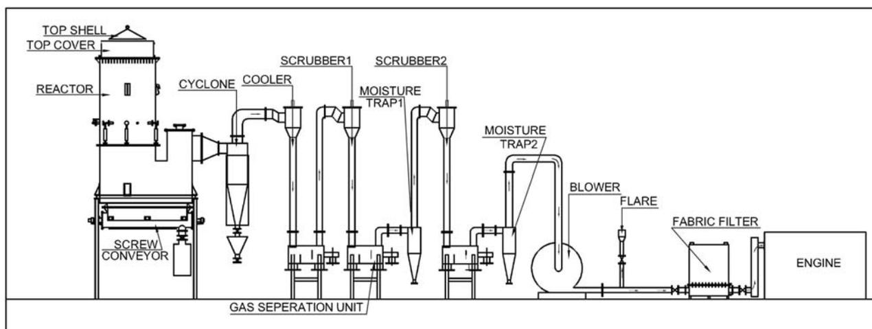
**Fig. 1** Schematic of the open-top down-draft gasification system
